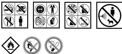
**DANGER** **Danger of death due to fire and/or explosion!** Danger of death due to improper use of the device! Avoid having sources of ignition in the surrounding area. For this reason, observe the following safety instructions:
