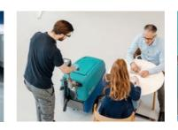
Whisper-quiet cleaning Noise reduction to 60db(A) thanks to the sound-insulated suction motors enables economical cleaning of highly frequented and noise-sensitive areas without any loss of performance.
